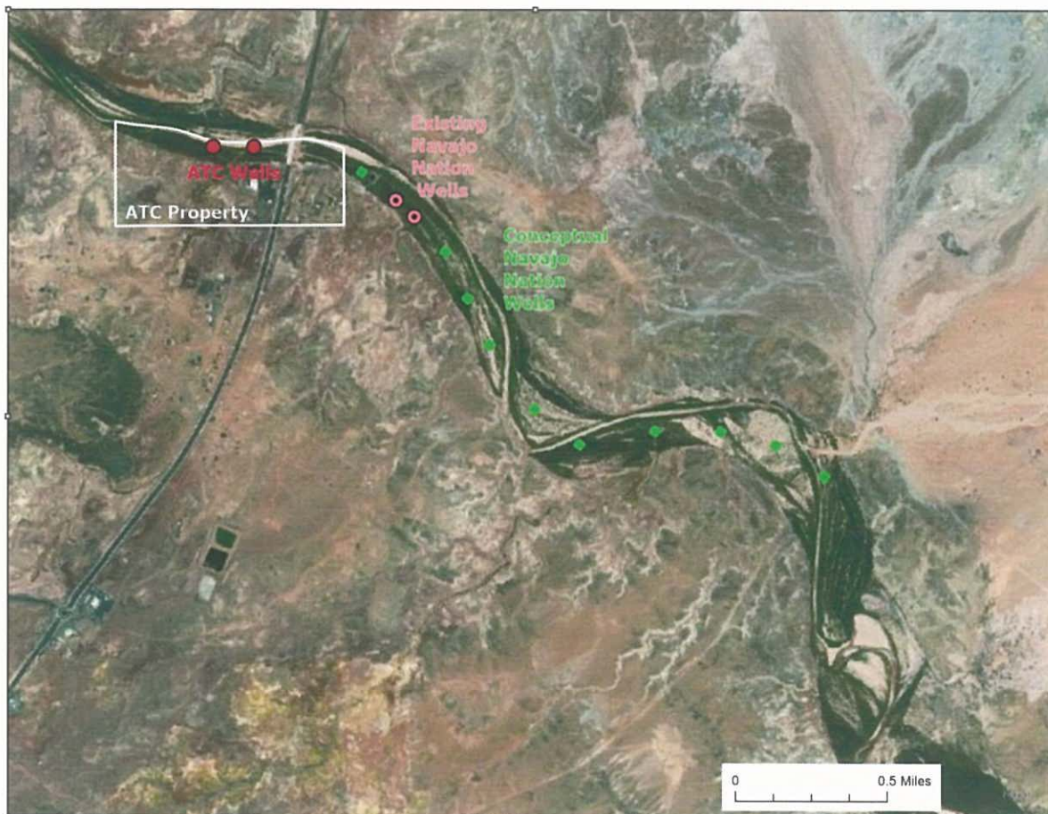
Figure 7. Example Navajo Nation wellfield layout for Scenario 3.
