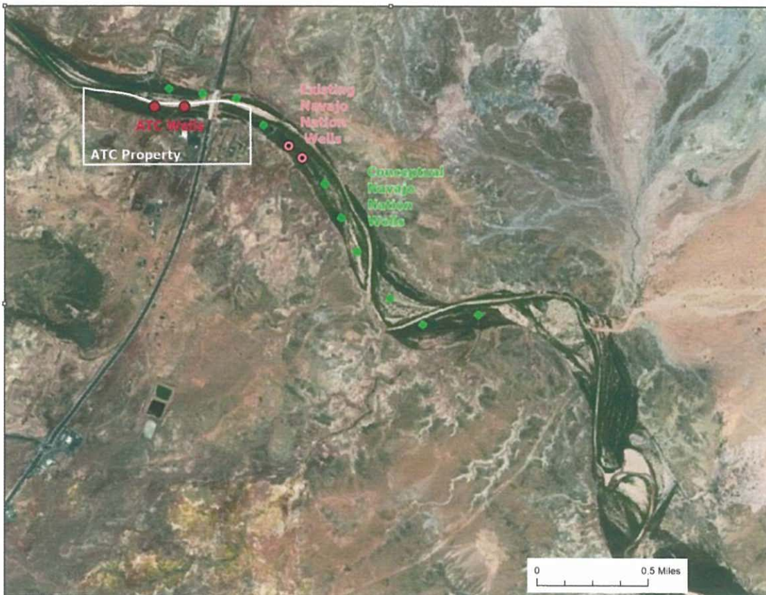
Figure 5. Example Navajo Nation wellfield layout for Scenario 1.
