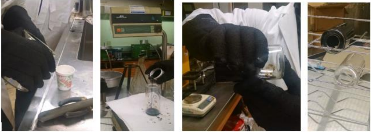
FIGURE 22 Sample preparation for RTFO test
