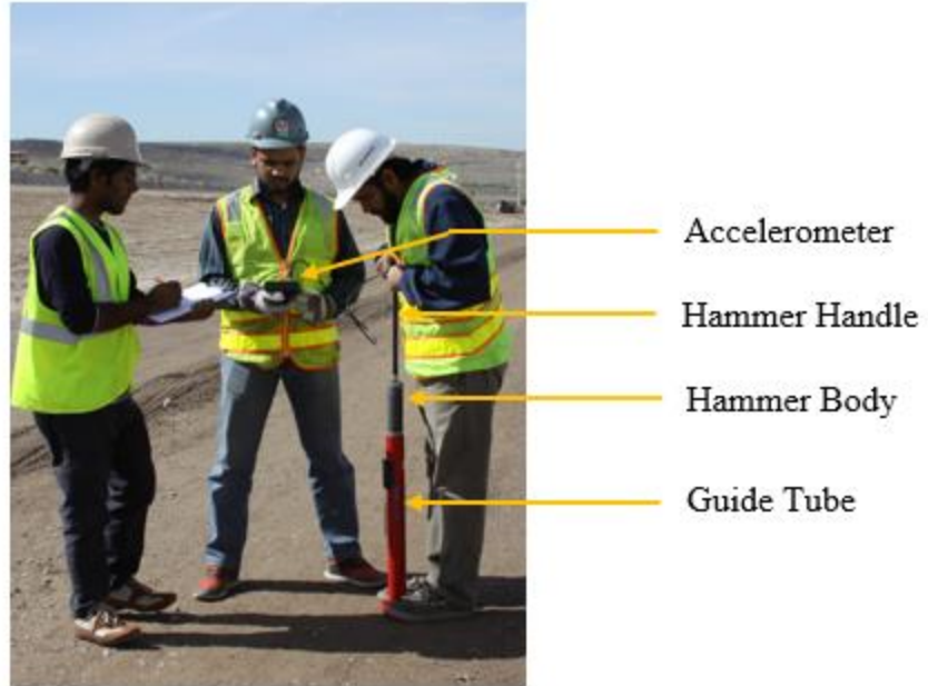
FIGURE 40 CIH testing device
