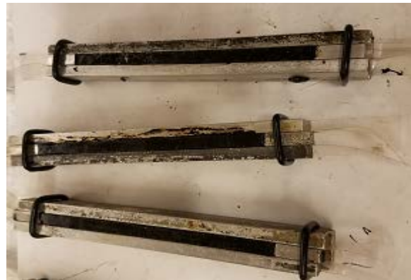
b) Asphalt binder beam samples
