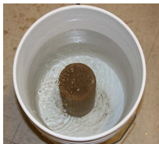
Figure 4.10: Soaked Soil Sample
