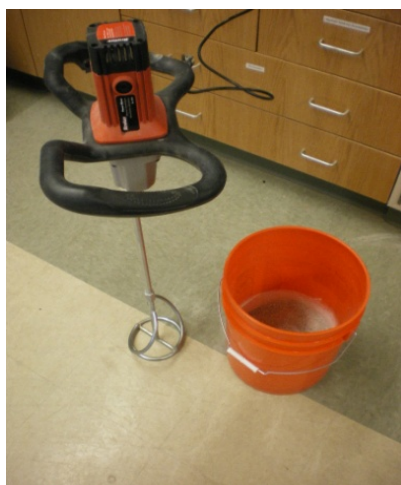
Figure 3.3 : Soil Mixing in Bucket Using Mechanical Mixer
