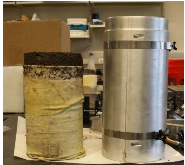
2.8" and 4" diameter subgrade soil mold 6" diameter base soil mold with compacted soil
