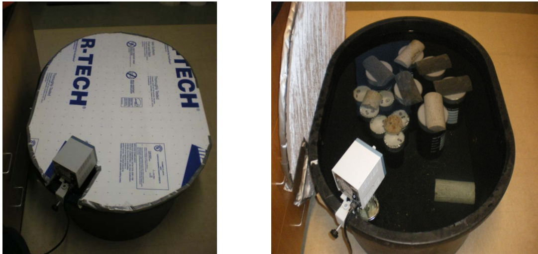
Figure 4.3: Stabilized Subgrade Soil in the Curing Tank
