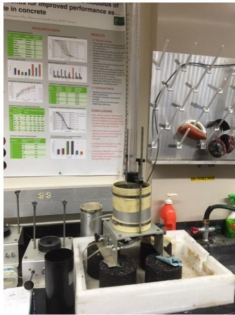
FIGURE 35 Permeability test setup
