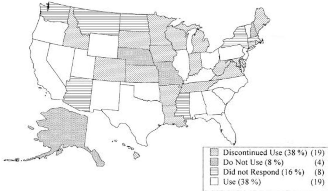
FIGURE 2 Use of OGFC by US states according to a survey by Kandhal and Mallick (2)
