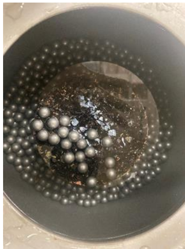
e) Specimen and steel charges are in container
