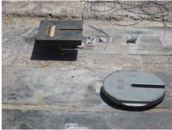
FIGURE 12 Weights Applied on Top of Each Installed Strain Gauge.
