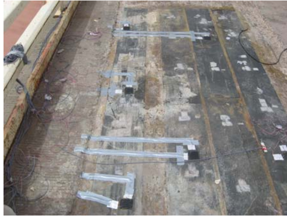
FIGURE 14 All the Strain Gauges After Being Installed on the FRP Sheets and Connected to the Wires Transmitting the Strain Signals to the Data Acquisition (DAQ) Device.
