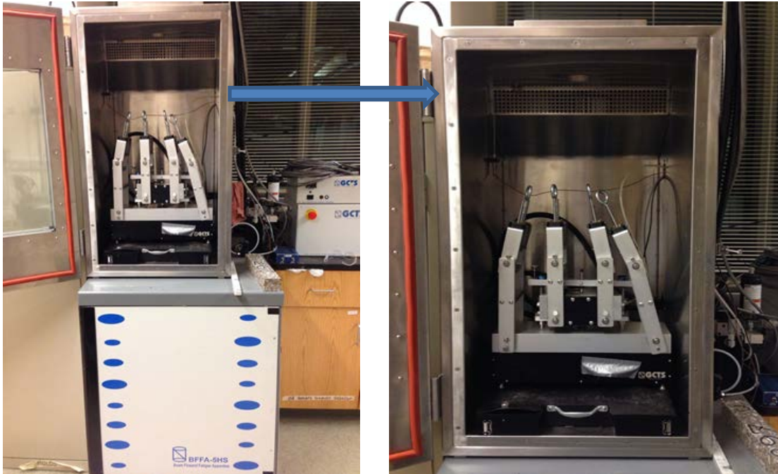
FIGURE 58 Beam Flexural Fatigue Apparatus by GCTS Testing Systems.
