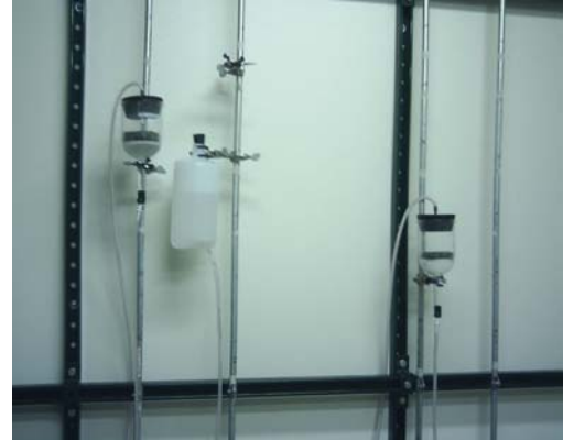
4.1(a) Hanging Column Test Setup
