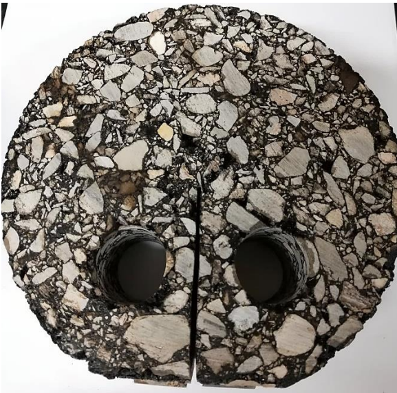
(a) A prepared sample for DCT test
