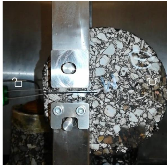
(b) DCT test in progress
