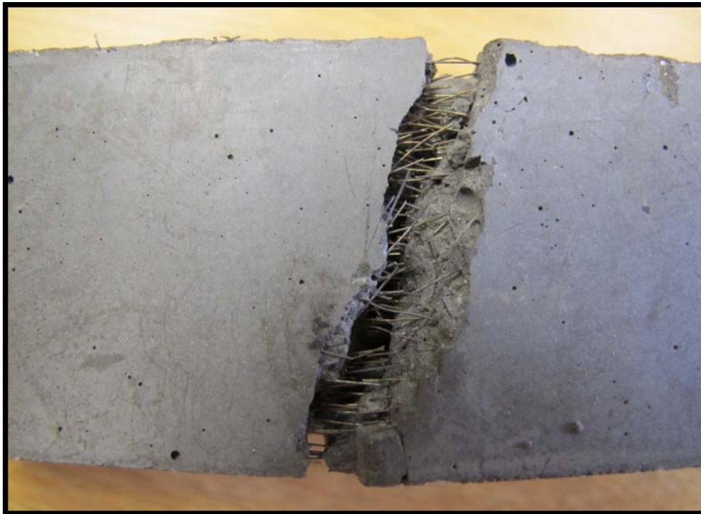
FIGURE 3.10 Close View of Crack Bridging Fibers in Test Prism.
