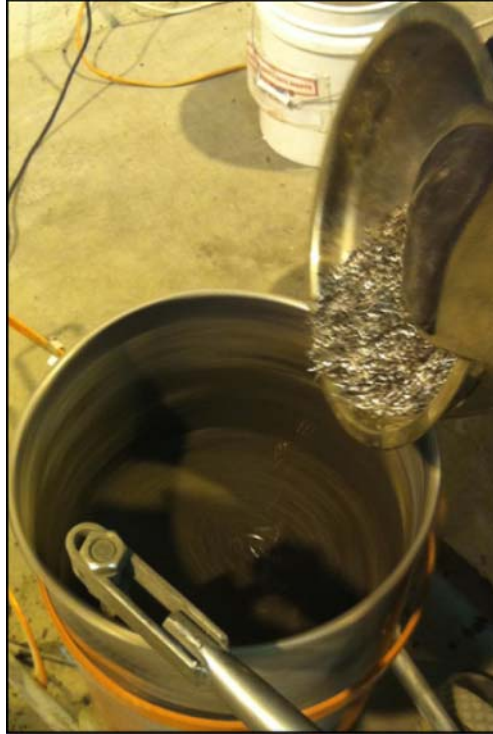
FIGURE 13.2 Photograph of steel fibers being added to slurry.
