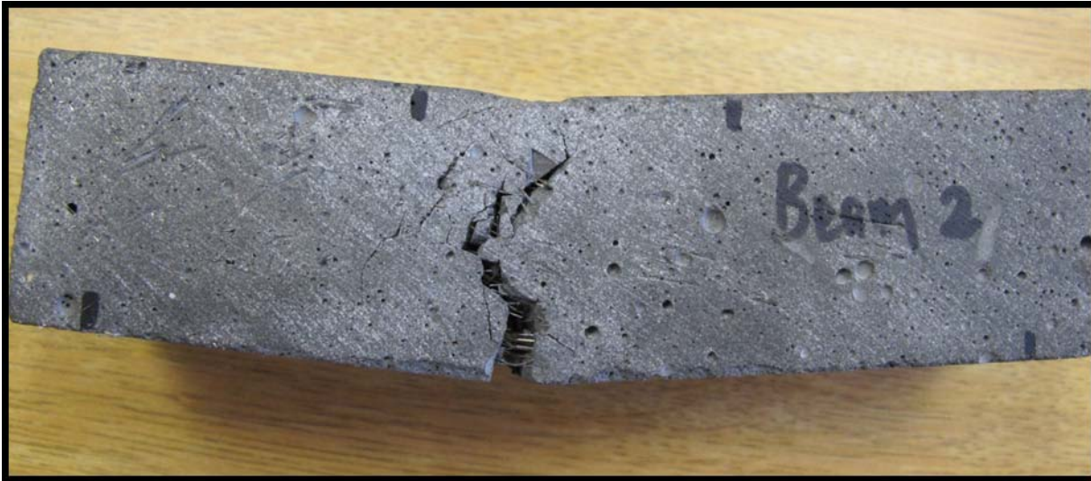
FIGURE 3.9 Test Prism from Flexural Testing of Mars Hill Bridge.
