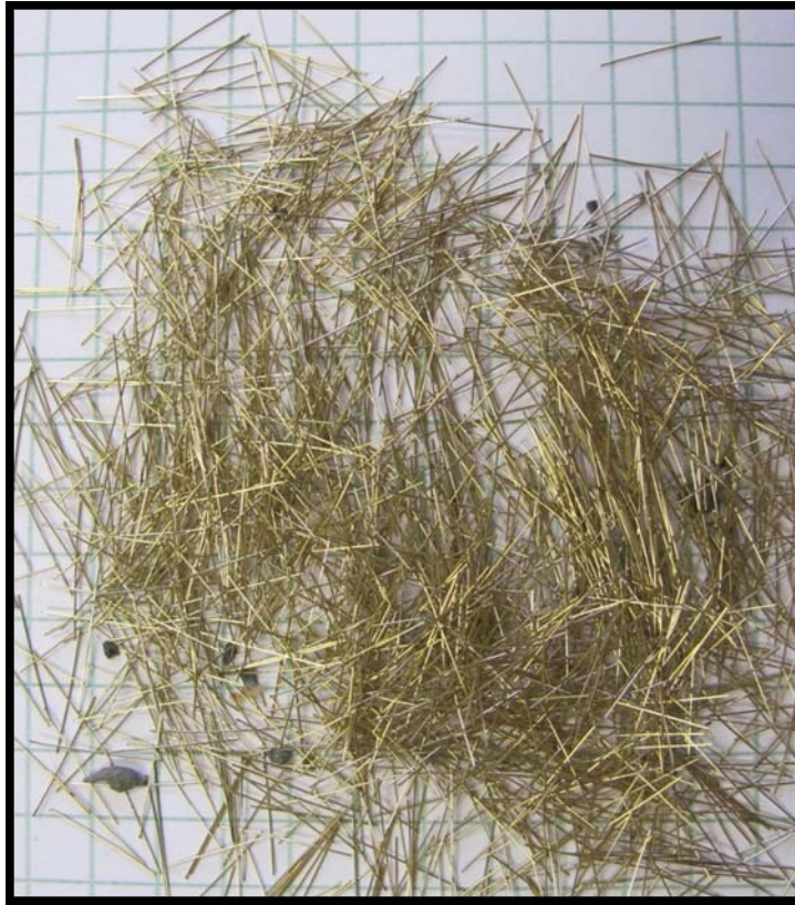
FIGURE 3.11 Sample of 0.5 in. (12 mm) Steel Fibers Used in UHPC Mix for Mars Hill Bridge.
